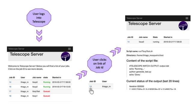
Telescope user interface: The first screen displays the status of the jobs on the cluster. The next screen shows detailed information about the first listed job: source directory, name and content of the script file, and last lines of current task output. Credit: Brito et al.
