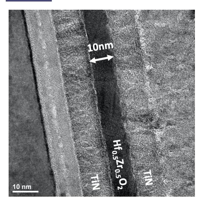
Transmission electron microscope image of the resonator's cross-section, highlighting the 10nm-thick ferroelectric Hf0.5Zr0.5O2 film sandwiched between 10nm-thick titanium nitride (TiN) electrodes. Credit: Ghatge et al.
