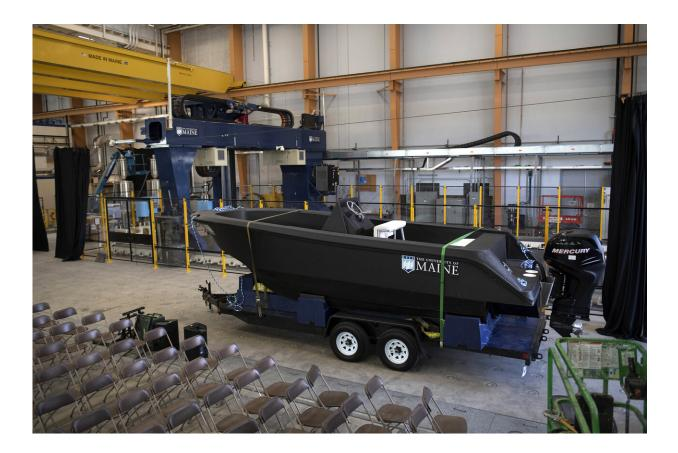
In this Wednesday, Oct. 9, 2019 photo provided by the University of Maine, a 25-foot, 5,000-pound patrol boat, center, that was produced using a large polymer 3D printer, behind left, rests on a trailer on the school's campus, in Orono, Maine. The boat was printed at the school's Composites Center on the world's largest polymer 3D printer. (Ron Lisnet/University of Maine via AP)
