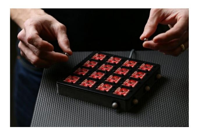
Two permanent magnets are tracked with magnetic field sensors. MIT engineers have devised an algorithm for high-speed tracking of any number of magnets, with significant implications for augmented reality and prosthesis control. Credit: Jimmy Day/MIT Media Lab and IEEE Sensors Journal/IEEE
