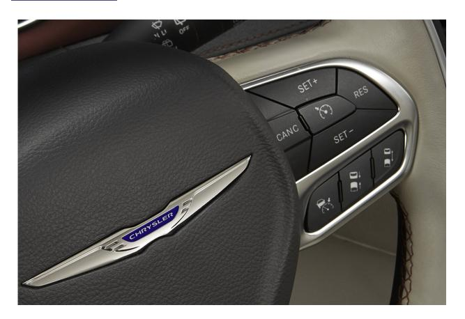
This undated photo provided by Chrysler shows the steering-wheel-mounted controls for the Pacifica minivan's adaptive cruise control. (FCA US via AP)
