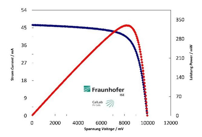
Measurement of the organic record solar module performed by the independent certification laboratory of Fraunhofer ISE (Freiburg). Credit: Forschungszentrum Juelich
