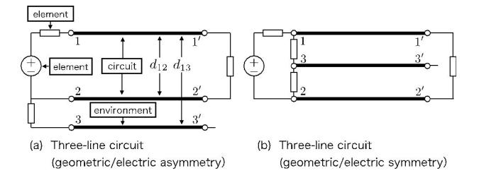
Figure 1. Three-line circuit configurations used in this study, which consider the environment around the electrical circuit (a) Geometrically asymmetric structure / electrically asymmetric connection (b) Geometrically symmetric structure / electrically symmetrical connection. Credit: Osaka University
