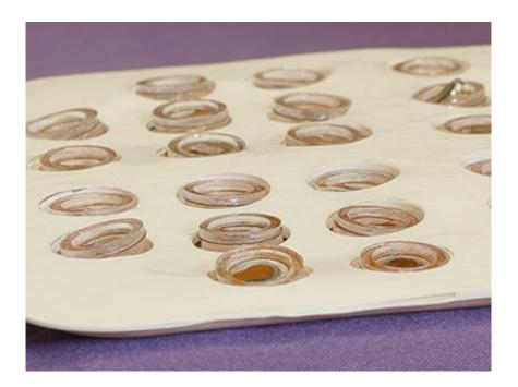
The 15-centimeter-by-15-centimeter sheet-like prototype can comfortably laminate onto the curved surfaces of the skin without bulky batteries and cumbersome wires. It holds 32 miniaturized actuators, embedded into soft, flexible silicone. Credit: Northwestern University
