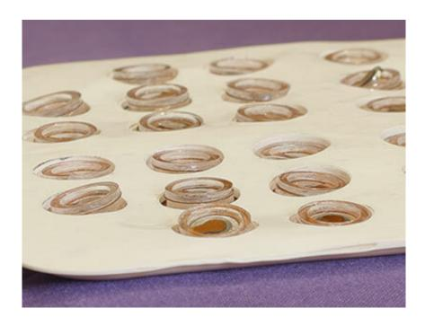
The 15-centimeter-by-15-centimeter sheet-like prototype can comfortably laminate onto the curved surfaces of the skin without bulky batteries and cumbersome wires. It holds 32 miniaturized actuators, embedded into soft, flexible silicone. Credit: Northwestern University
