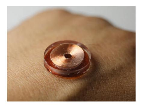
The single, miniaturized actuators measure just 18 mm in diameter and 2.5 mm thick. Each actuator resonates most strongly at 200 cycles per second, where the skin exhibits maximum sensitivity. Credit: Northwestern University
