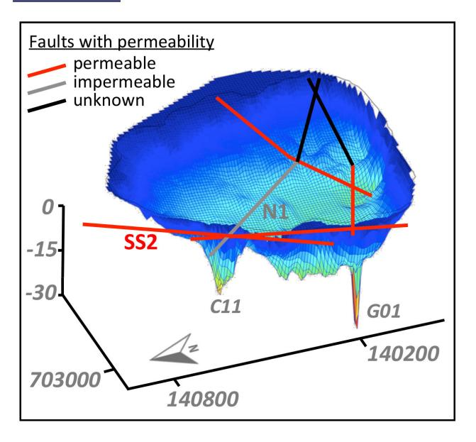
3D representation of the lake depth with fault zones running through the lake. Points G01 and C11 show geyser-like holes through which hot water is carried into the lake. Credit: CC BY 4.0: Maren Brehme; DOI:10.1038/s41598-019-52638-z
