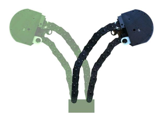
The new "growing robot" can be programmed to grow, or extend, in different directions, based on the sequence of chain units that are locked and fed out from the "growing tip," or gearbox. Credit: Massachusetts Institute of Technology
