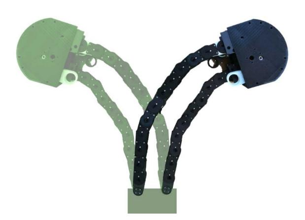
The new "growing robot" can be programmed to grow, or extend, in different directions, based on the sequence of chain units that are locked and fed out from the "growing tip," or gearbox. Credit: Massachusetts Institute of Technology
