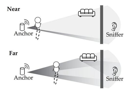
Illustration shows how inexpensive devices can turn Wi-Fi signals into motion detectors. Credit: University of Chicago
