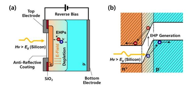
(a) A schematic of simple PN junction photodiode, (b) PN junction photodiode internal band diagram when light source is incident. Credit: Kim et al.
