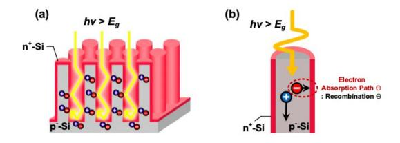
(a) Low surface reflectance in the SiNW array, (b) separation of absorption path between light and electrons. Credit: Kim et al.
