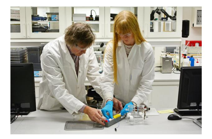
Researchers Odne Stokke Burheim and Kjersti Wergeland Krakhella assemble the membrane conductivity measurement cell they used to test their use of waste heat to help produce hydrogen. Photo: Lars Robert Bang/NTNU
