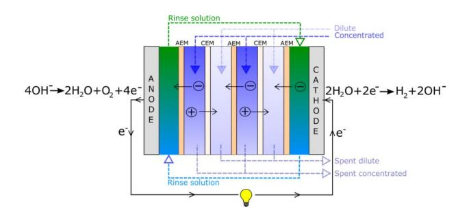
Here's a visualization of what a RED cell looks like. The hydrogen is produced at the cathode end and oxygen is produced at the anode end. Illustration: NTNU
