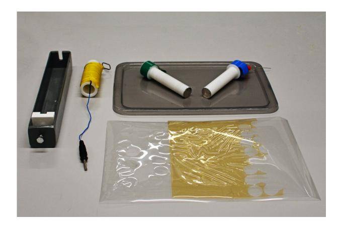
Here's what it takes to make the cells. In the front of the picture is the ion exchange membrane, while in the back are the cell components used to measure the membrane conductivity. Photo: Lars Robert Bang/NTNU
