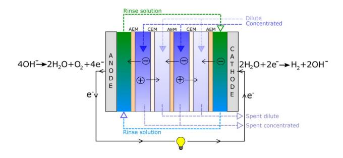
Here's a visualization of what a RED cell looks like. The hydrogen is produced at the cathode end and oxygen is produced at the anode end. Illustration: NTNU
