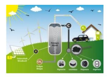
Methane pyrolysis by means of a bubble column reactor allows for the climate-friendly use of fossil natural gas. Credit: Leon Kühner, KIT
