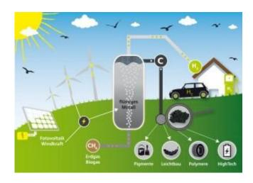
Methane pyrolysis by means of a bubble column reactor allows for the climate-friendly use of fossil natural gas. Credit: Leon Kühner, KIT
