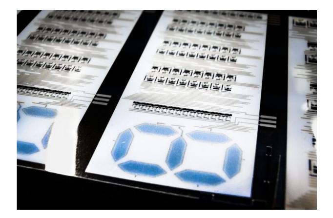
These large-scale integrated circuits, LSI, can be used, for example, to power an electrochromic display, itself manufactured as printed electronics. Credit: Thor Balkhed
