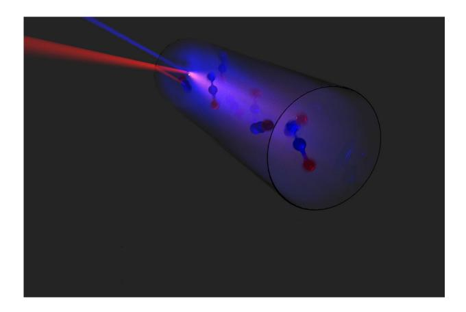
Artistic view of the QCL pumped THz laser showing the QCL beam (red) and the THz beam (blue) along with rotating N2O (laughing gas) molecules inside the cavity. Credit: Arman Amirzhan/Harvard SEAS
