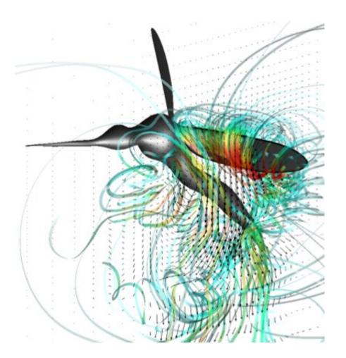
Complex streamlines generated by the flapping wing of a mosquito in flight. Mosquitoes flap their wings not just to stay aloft but for two other critical purposes: to generate sound and to point that buzz in the direction of a potential mate, researchers at Johns Hopkins University have discovered. Credit: Rajat Mittal
