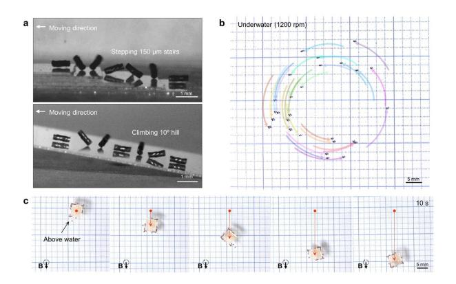
Hierarchical magnetomotility driven by rotational and revolving movements of helical magnetic soft robots permits (a) climbing over obstacles, (b) underwater swimming of multiple soft robots, and (c) collective transportation of cargo via a single rotating axis of permanent magnets. Credit: Inha University
