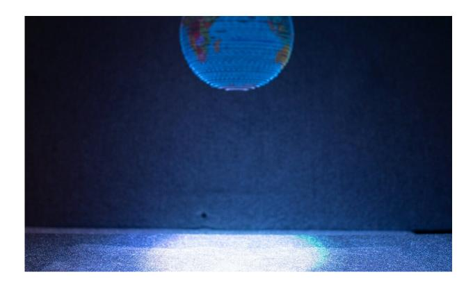
Globe created by the Multimodal Acoustic Trap Display developed at the
