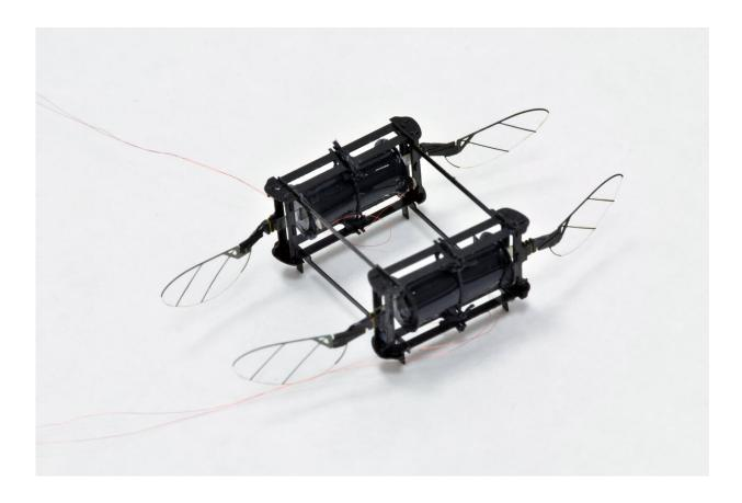
A four-wing, two actuator model could fly in a cluttered environment, overcoming multiple collisions in a single flight. Credit: Harvard Microrobotics Lab
