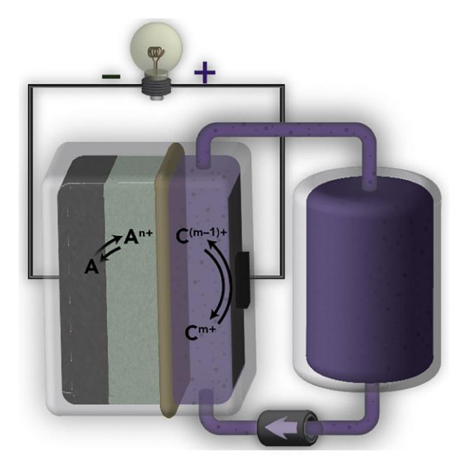
Schematic of a flow battery with an ion-selective AquaPIM membrane (noted in beige). Berkeley Lab scientists discovered that such a model could predict the lifetime and efficiency of a flow battery for the electric grid without having to build an entire device. Credit: Brett Helms/Berkeley Lab
