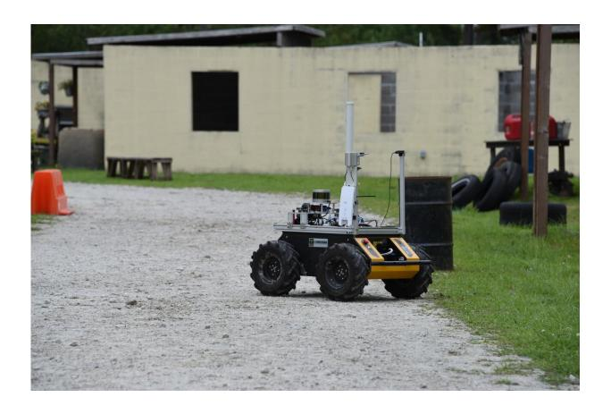
The Clearpath Husky, used as a research platform, is used to develop and test underlying autonomy to support context-driven AI that supports effective bidirectional communication. Credit: ARL
