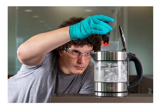
Microsoft Project Silica researcher Youssef Assaf drops a square of silica glass in a kettle of boiling water to demonstrate its durability. The team has baked, boiled, microwaved, demagnetized and scoured similar pieces of glass with steel wool — with no loss to the data stored inside. Credit: Jonathan Banks for Microsoft.
