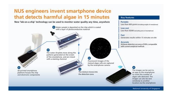
The smartphone device can generate test results on-site, and findings can be reported in real-time. Credit: National University of Singapore
