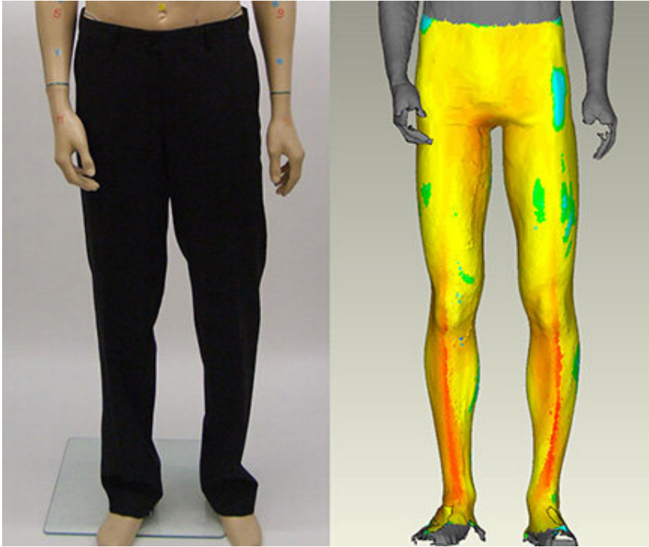
Example of garments and the air layers that form underneath. Credit: Empa
