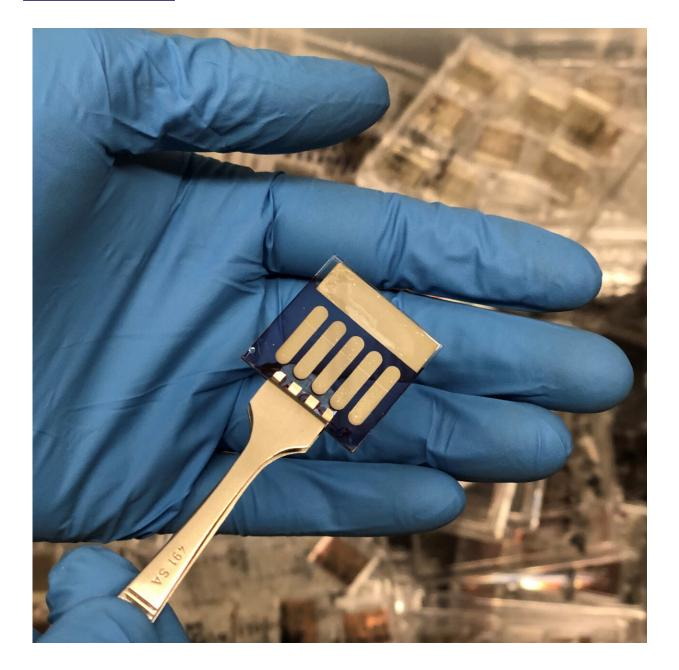
This sample includes five small area organic photovoltaic devices that were fabricated in the Kippelen Research Group at Georgia Tech. Samples with similar geometry were sent to the ISS to investigate the effects of exposure to space environments. Credit: Bernard Kippelen, Georgia Tech
