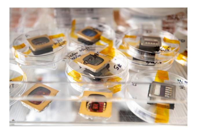
Selection of solar cells in the laboratory of GTRI Principal Research Engineer Jud Ready. The cells include 3D, CZTS, organic photovoltaic, and silicon. Credit: Branden Camp, Georgia Tech
