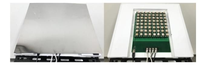
Fig. 3. StickyTouch covered with a stainless-steel plate (left) and StickyTouch uncovered (right). Credit: Osaka University
