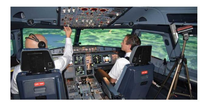
In the cockpit of an A320 flight simulator, an eye-tracking system consisting of cameras and infrared sensors keeps constant track of where the pilot (left) is looking. Credit: David Rudi/ETH Zurich
