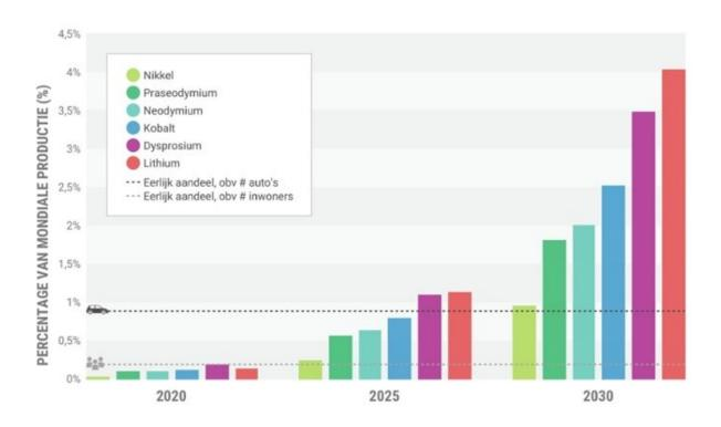
Figure 1. Critical metals needed for electric vehicles in the Netherlands, as a percentage of the worldwide annual production of these critical metals in 2020, 2025 and 2030. Credit: Leiden University
