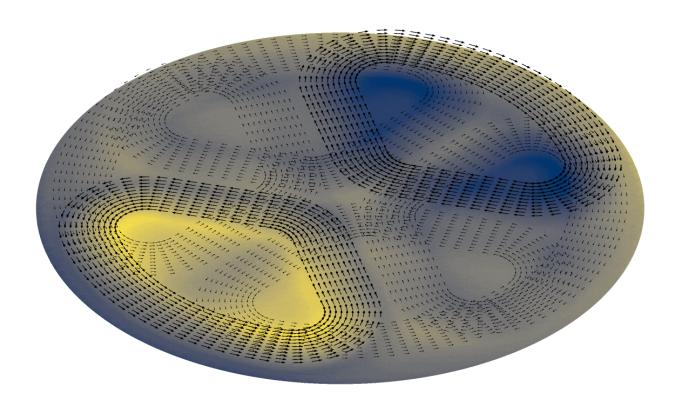
New wireless charging coil designs, created and tested by Oak Ridge National Laboratory, include a three-phase system that features rotating magnetic fields between layers of coils. The layered coils transfer power in a more uniform way, allowing for an increase in power density. Credit: Jason Pries/Oak Ridge National Laboratory, U.S. Dept. of Energy
