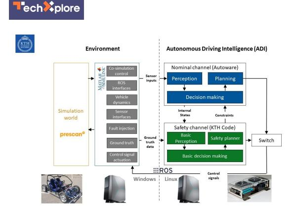
Figure outlining the structure of the simulation platform. Credit: Mohan & Törngren.
