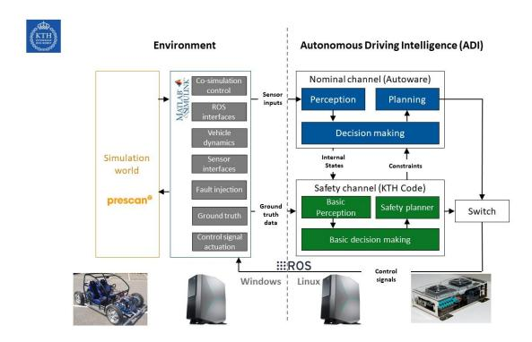
Figure outlining the structure of the simulation platform. Credit: Mohan & Törngren.
