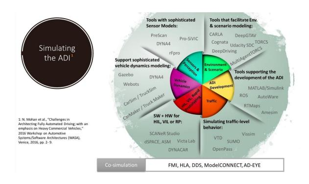
Figure summarizing some of the tools for simulating automated driving. Credit: Xinhai Zhang.
