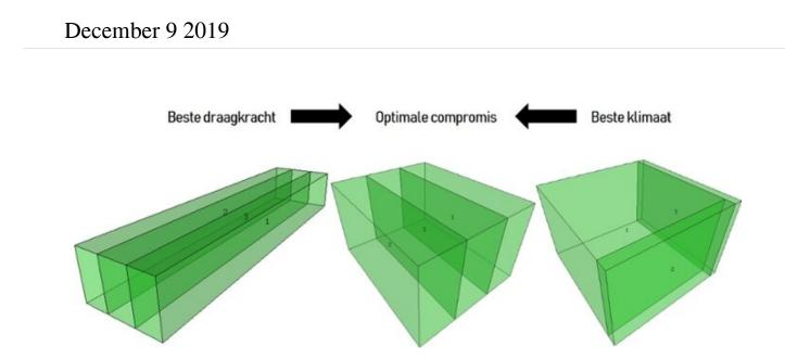
Van der Blom: "You can imagine that the smaller the surface area of the outer walls, the less heat you lose or get inside. In other words: the more the building looks like a cube, the less external influence. However, for the load-bearing capacity, a more elongated building is better, in which the span of the roof between two walls is as small as possible." Credit: Leiden University
