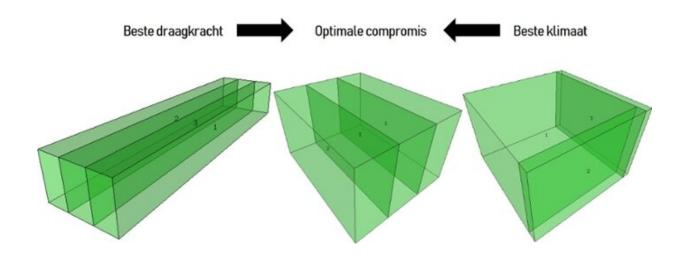
Van der Blom: "You can imagine that the smaller the surface area of the outer walls, the less heat you lose or get inside. In other words: the more the building looks like a cube, the less external influence. However, for the load-bearing capacity, a more elongated building is better, in which the span of the roof between two walls is as small as possible." Credit: Leiden University
