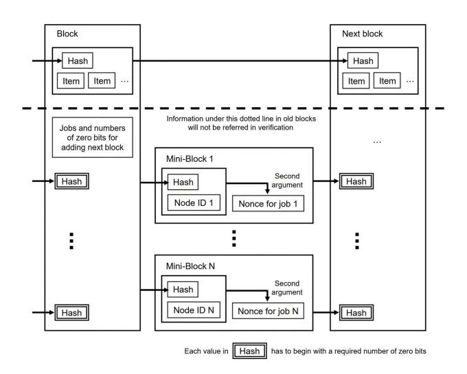
The data structure of a block in a blockchain with the proposed protocol. Credit: Naoki Shibata
