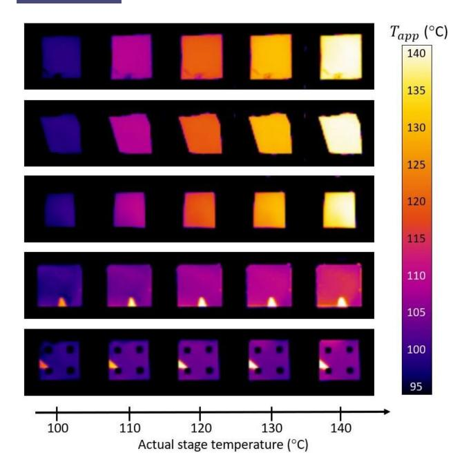
Infrared images show conventional materials (top three rows) appear to an infrared camera as they heat up. Special coatings developed by UW–Madison engineers hide the temperature changes of the objects in the bottom two rows. Credit: Patrick Roney, Alireza Shahsafi And Mikhail Kats
