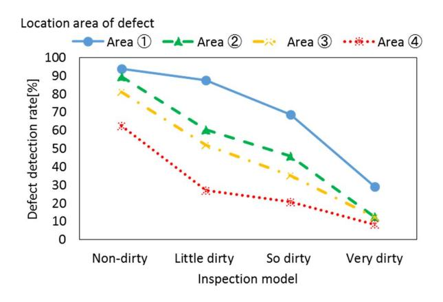
Relationship between dirt levels of inspection surface and defect locations. Credit: University of Electro-Communications
