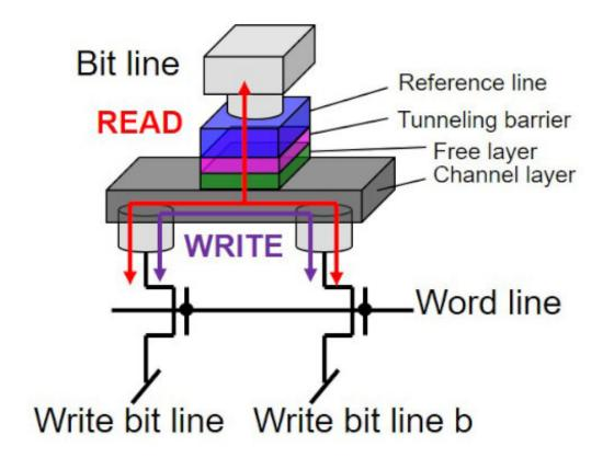
A schematic of the SOT-MRAM cell (Three Terminal Device) Credit: CIES, Tohoku University
