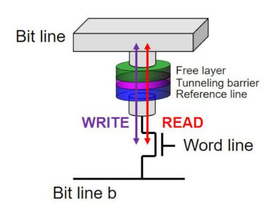
Schematic of STT-MRAM cell (Two Terminal Device). Credit: CIES, Tohoku University
