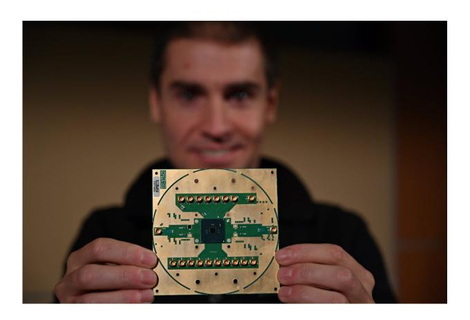
Stefano Pellerano, principal engineer at Intel Labs, holds Horse Ridge. The new cryogenic control chip will speed development of full-stack quantum computing systems, marking a milestone in the development of a commercially viable quantum computer. Credit: Walden Kirsch/Intel Corporation
