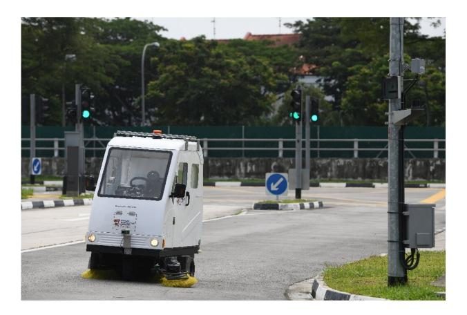
The test site has a track with sharp turns, traffic lights, a slope, and a bus stop to simulate real driving conditions
