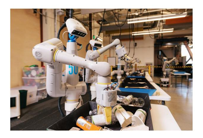
Robots sorting compost, recycling, and landfill waste at our offices as part of our sorting experiment. Credit: Alphabet X
