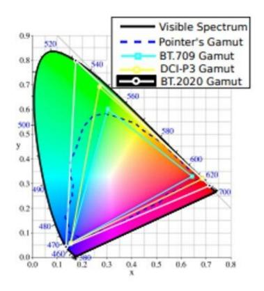
The range of colours that a device can reproduce is called a gamut. A very common and convenient way of describing colours is to ignore their luminance component and represent only the chromatic content in a 2D plane known as the xi CIE chromaticity diagram. Credit: UPF
