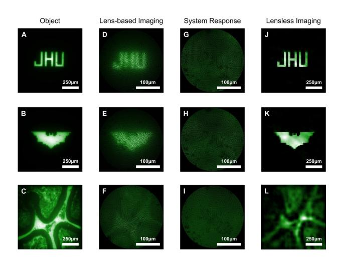
A to C shows beads on a slide imaged by a bulk microscope. D to F are the beads when viewed from a conventional lens-based microendoscope. G to I are the raw images from the research team's new ultra-miniaturized lens-free microendoscope. The researchers say these images are terrible but actually provide a great deal of information about light coming through that can be used in computational reconstruction to piece together a clearer final image. J to L are
