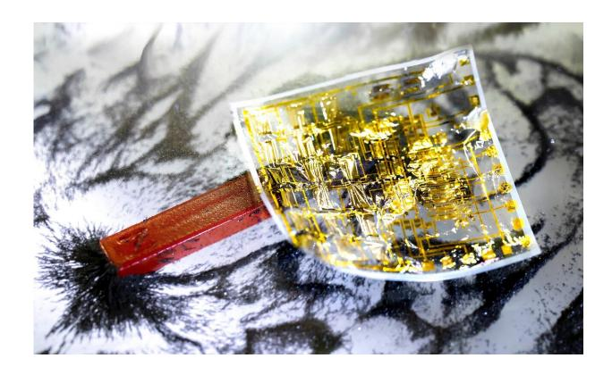
Flexible electronic skin equipped with an array of giant magneto resistance sensors and complex electronics circuit designed and developed for sensing distribution of magnetic field. Credit: Masaya Kondo
