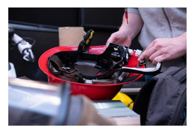
Firefighters don't need extra time to put on the helmet because the haptics are embedded inside the prototype. Credit: Carnegie Mellon Engineering
