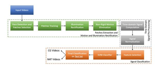
Algorithm process flow. Three main phases characterize the workflow: (a) temporal signal computation from face patches and denoising; (b) signal normalization; and (c) feature extraction and SVM classification. Credit: Bonomi and Boato
