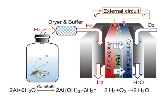
A schematic diagram demonstrating the combination of a hydrogen extraction system and a PEMFC for power supply. Credit: Jing Liu
