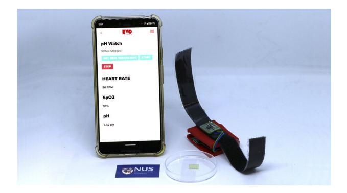
By integrating the NUS team's custom-made pH sensor (middle) and pH sensing algorithm into existing fitness trackers or smartwatches which already have a built-in pulse oximeter, the pH Watch can simultaneously monitor the pH value of a user's sweat, along with heart rate and blood oxygen saturation values in real-time, with about 90 per cent accuracy. Credit: National University of Singapore
