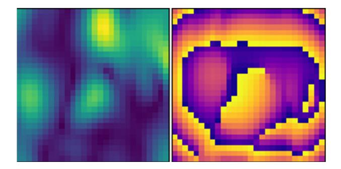
An example of a wave pattern (right) and its intensity levels (left) developed by the machine learning algorithm to best illuminate the most important features of an object being identified. Credit: Mohammadreza Imani, Duke University
