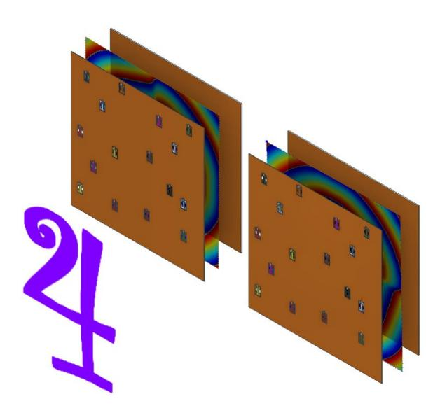
In a new type of object identification, a radio wave source (back panel) creates a wave front (middle panel) that is shaped by a metamaterial screen which allows waves to pass through in some places but not others (front panel). Machine
