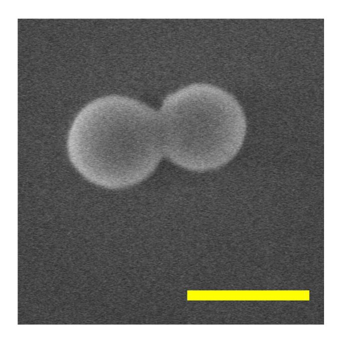
The fastest-spinning object ever created is a nano-scale rotor made from silica at Purdue University. This image of the rotor at rest was created using a scanning electron microscope. For scale, the yellow bar in the image is 200 nanometers.
