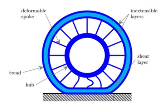
Illustration of a non-pneumatic tire structure showing the shear layer. Credit: University of Illinois at Urbana-Champaign
