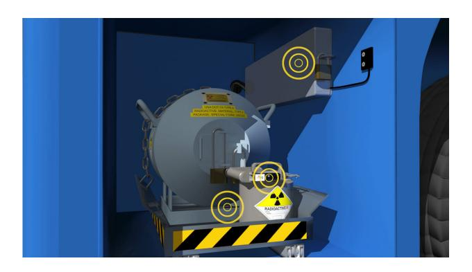
A well logging configuration for MSTS consists of radiation measurement devices, radiofrequency tags and other loss detection technology. MSTS, developed by PNNL, has been licensed to Golden Security Services. Credit: PNNL
